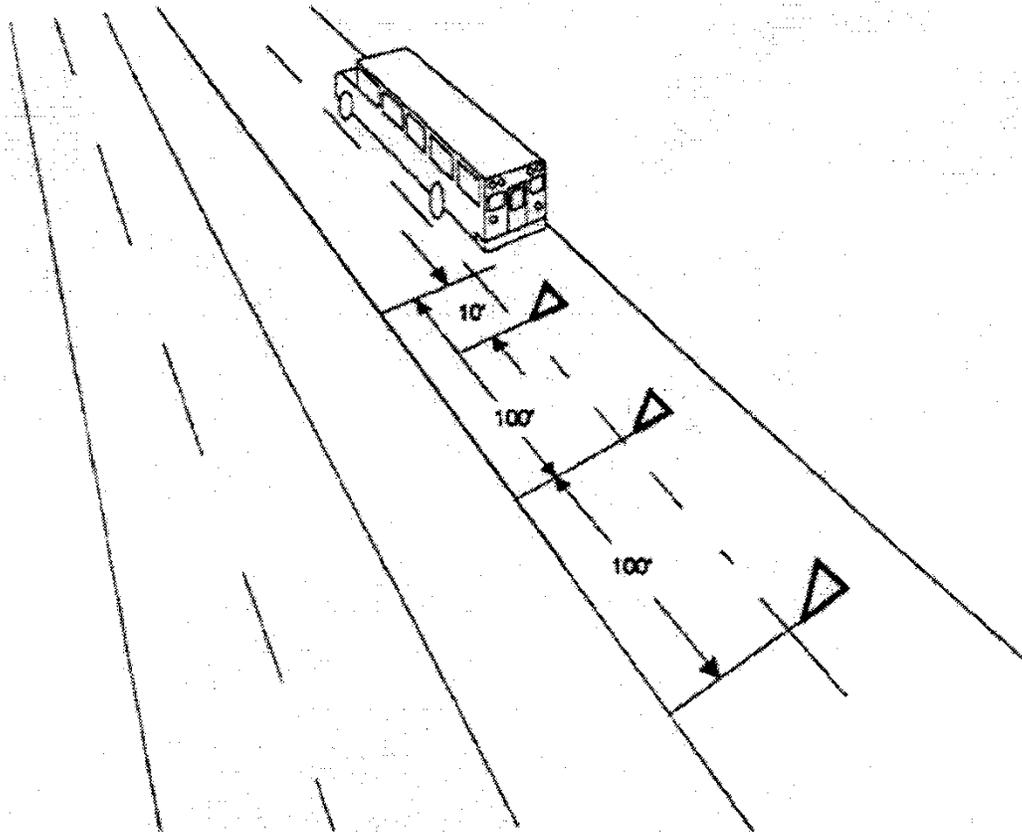
When placing the triangles, hold an assembled triangle toward the oncoming traffic. This enhances safety by increasing visibility to other drivers (especially at night).
