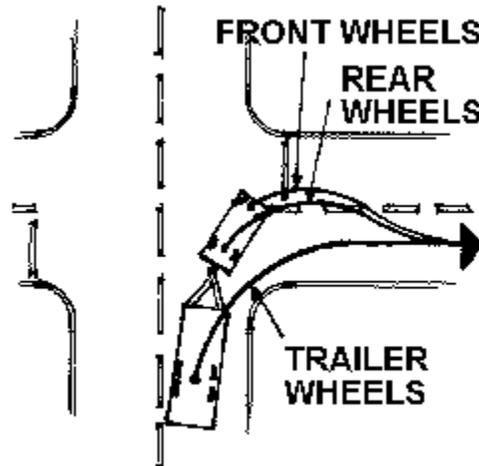
*The longer the trailer, the wider you must swing in a turn to make sure the trailer wheels clear the inside curb.*
