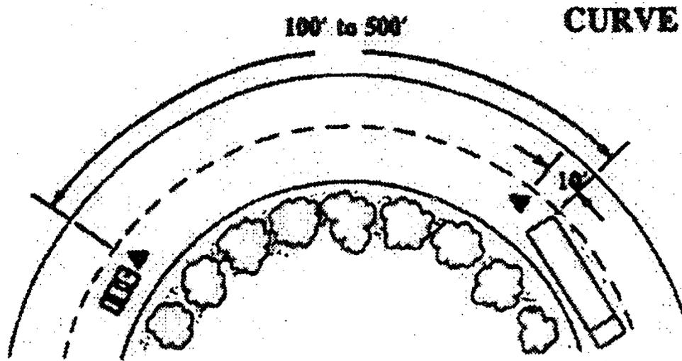
*Reminder: If the line of sight is obstructed due to a hill or curve, move the rearmost triangle to a point giving adequate warning.*
