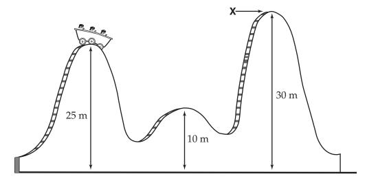
The car on the roller coaster is released from the position shown and allowed to roll freely.
