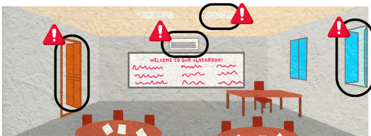
Figure 8: Common causes of noise in a classroom can include open doorways to public areas, open windows, HVAC systems, and more.
