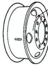
Cracks at disc nave
