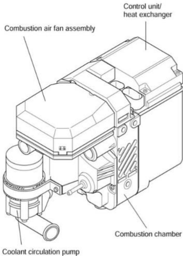
**Figure 1. TSL 17 (Thermo Top C) Coolant Heater**
