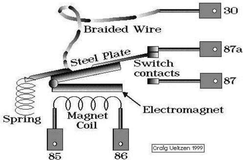
Relays are used to transfer high current. When power is applied across the 85 and 86 terminals, current flows through a coil of small wire. This builds up a magnetic field in the bar it's wrapped around, and the steel plate snaps to it. When the power is off, the spring pulls the plate back away from the magnet bar. The "click" is the plate slamming into the magnet as it turns on. It doesn't "click" when turned off, because the plate swings away from the magnet without hitting anything.
