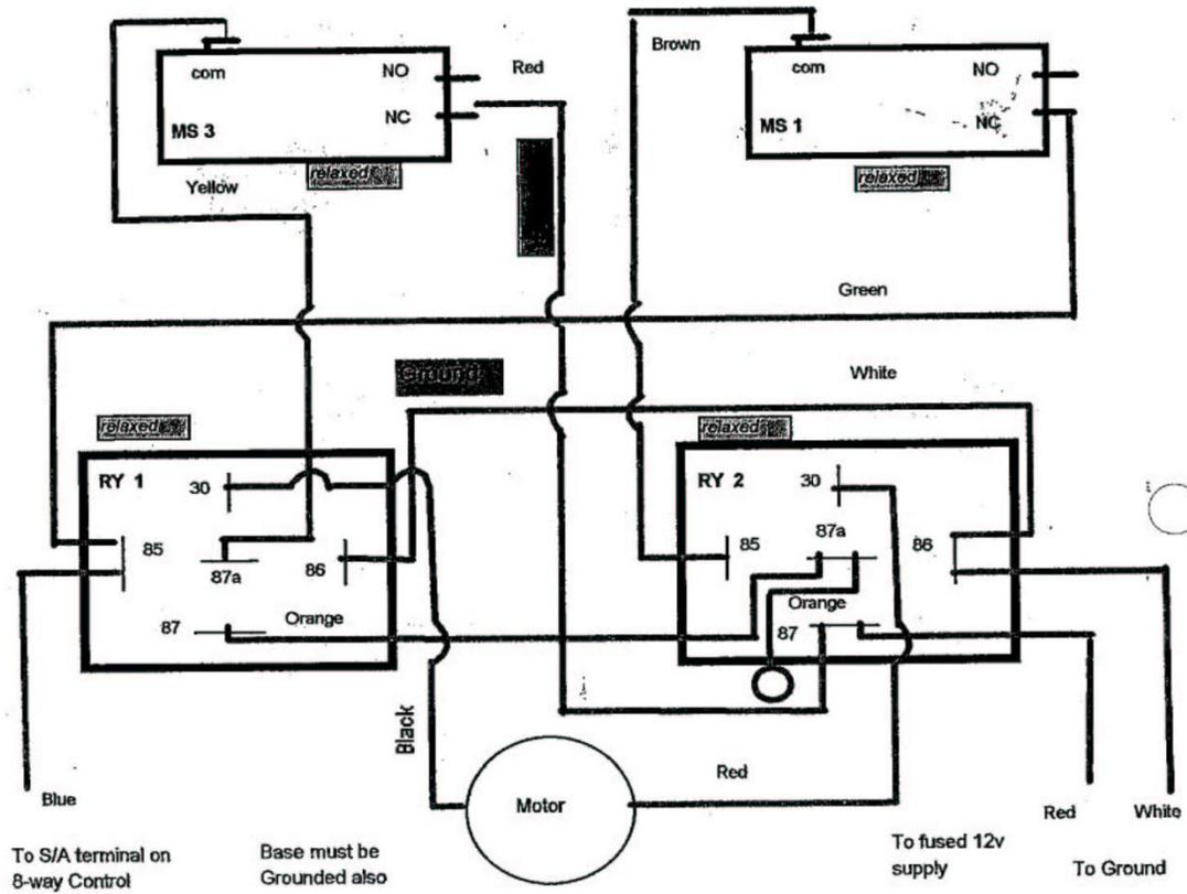
When the door is closed, the steady 12v signal disappears from the 8-way Control. All microswitches and relays become relaxed to apply 12v to the Black motor lead and ground to the Red motor lead. The motor runs to move the gate into the closed position as determined by MS3 and the whole cycle can start over!
