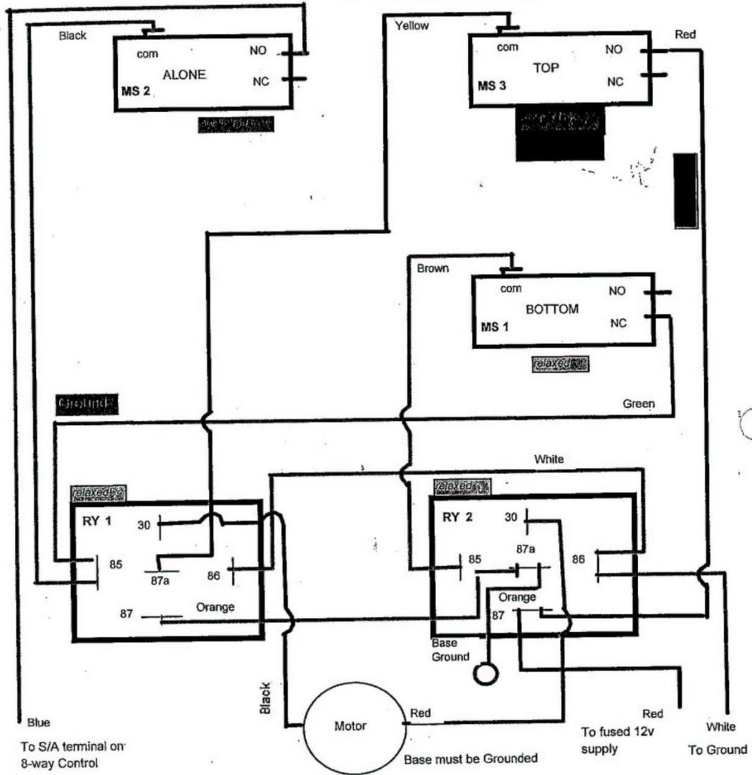
MS3 senses the proper closed position per the cam to be relaxed and thus both motor leads are at ground voltage. When the arm is not at the proper closed position, MS3 becomes switched and applies the 12v to the Black motor lead and the motor runs to bring the arm into the 0° position!
