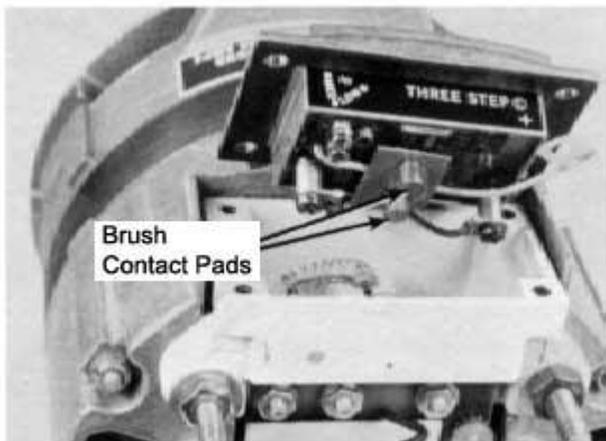
5. To adjust the voltage, remove and reinstall the adjustment strap in one of three positions: between terminals A and B (low), between terminals A and C (medium), or between terminals B and C (high). Each change in the strap will result in an increase
