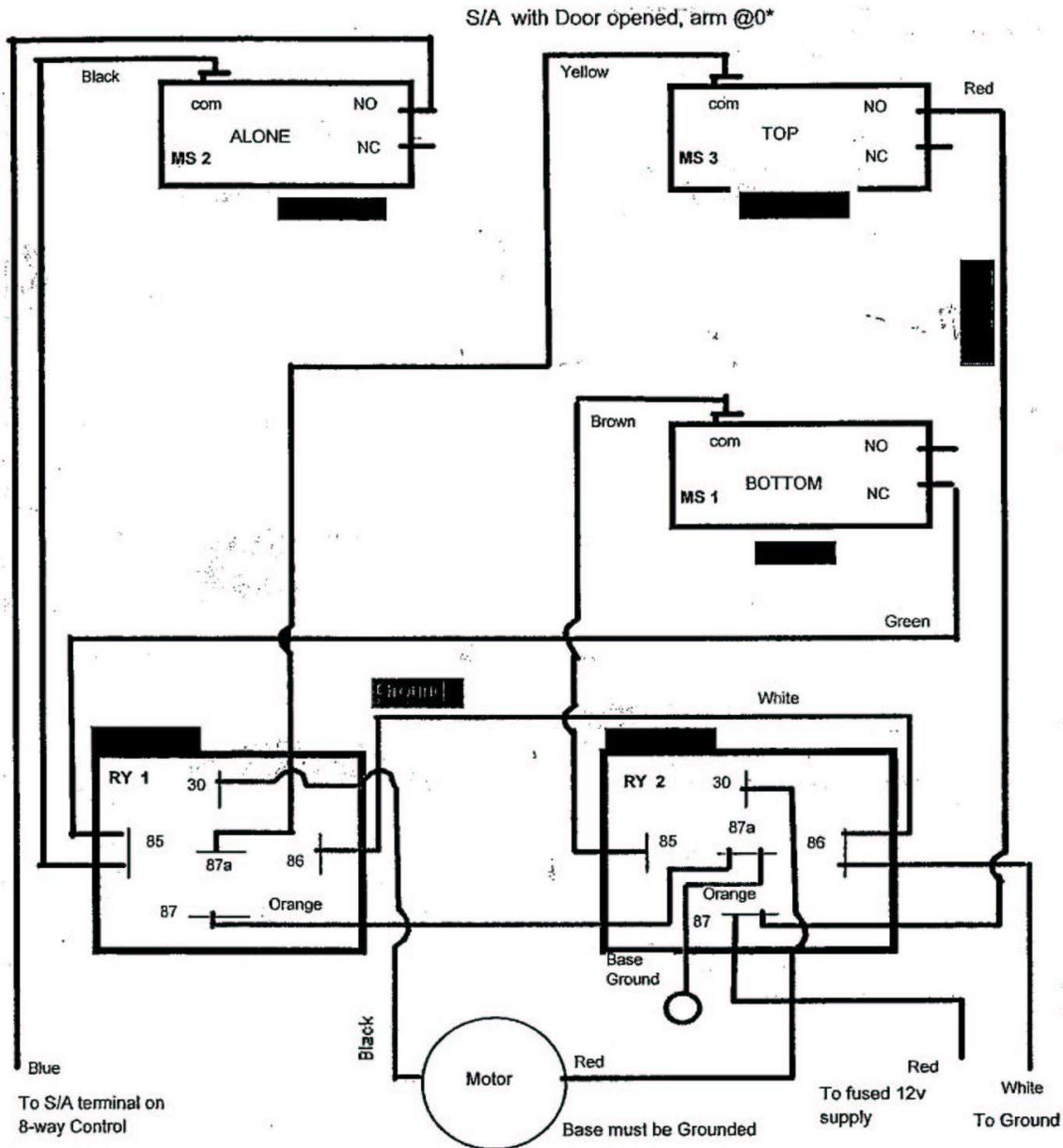
When the door is opened, the Blue wire from the 8-way Control becomes a steady 12v signal. This signal energizes both relays which reverses the voltage polarity on the motor leads resulting in the motor running to open the arm to the 90° position as determined by MS1 and the cam!
