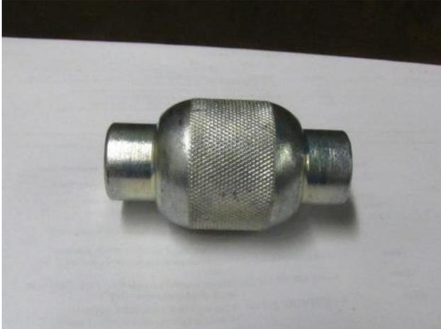
The anchor pins should be intact, with all the correct washers, springs, and spring washers in proper placement. Replace any pins, washers, springs, spring washers, snap rings, or C-clips that are damaged.
