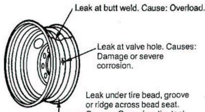
Leak at butt weld. Cause: Overload.
