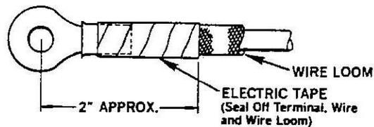
**Typical wire ending when replacing damaged wires or corroded terminals.**
